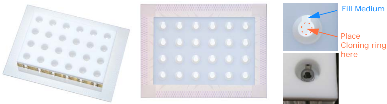
Figure 1-4. CellSpotter24-eco plated on the MEA 24well Plate-comfort (left, middle), and CellSpotter with cloning ring inserted (right).
