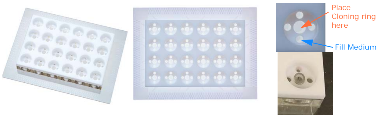
Figure 1-3. CellSpotter24-comfort placed onto the MEA 24well Plate-comfort (left, middle), CellSpotter24-comfort with cloning ring inserted (right).
